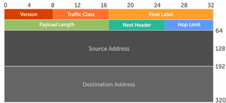
Figure 47. IPv6 Header Fields
